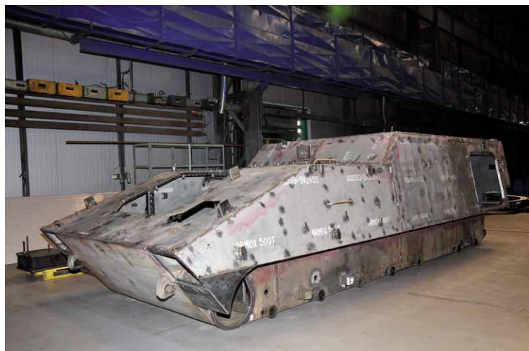
The hull of the Command & Control vehicle during machining.
